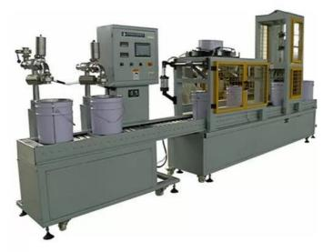
With its fast filling speed and precise measuring capabilities, the 1-10L drum fully automatic filling production line is suitable for a wide range of industries, including chemical, pharmaceutical, food and beverage, and oil and gas. The system can accurately fill drums of various sizes and shapes, making it a versatile solution for any manufacturing process.
