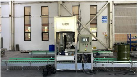
High Precision IBC Fully Automatic Vertica Ton Barrel Filling and Capping Machinery Machine for Solvent/Paint/Chemical/Lubricating Oil/Liquid
